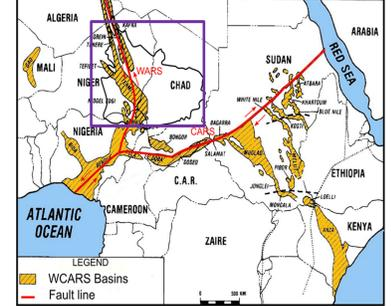
The WARS extension and its location. It is divided in WARS and CARS. The dotted lines indicate the general trace of East African Rifting, the solid red line represents the major fault, the dashed line means a probable fault. Image modified from Wycisk et al., 1990 and Genik, 1993 (\*\*)
