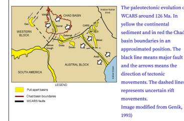
The paleotectonic evolution of WARS around 126 Ma. In yellow the continental sediment and in red the Chad basin boundaries in an approximated position. The black line means major fault and the arrows means the direction of tectonic movements. The dashed lines represents uncertain rift movements. Image modified from Genik, 1993
